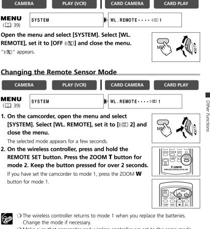
O Make sure that camcorder and wireless controller are set to the same mode. Display the camcorder's mode by pressing any button on the wireless controller (except of the REMOTE SET button) and set the wireless controller's mode to the same mode. Change the batteries if the wireless controller still does not work.
